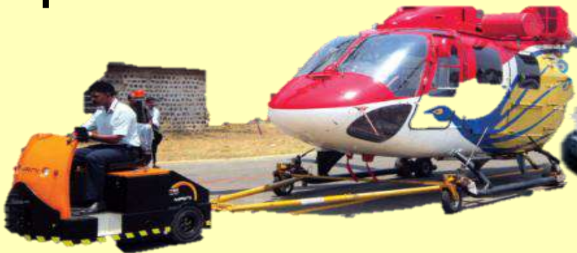
Electric Tow Truck towing helicopter
