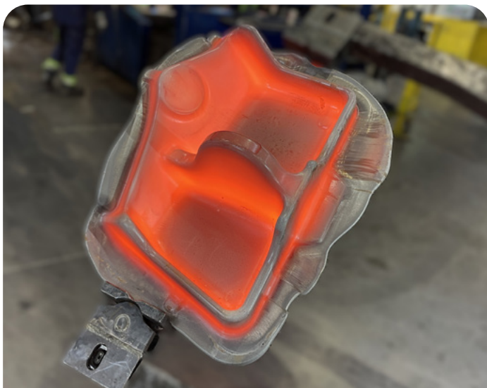
↓ Titanium forging for the Airbus A350, Otto Fuchs
