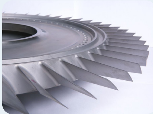
→ Integrated engine disk (blisk) for the Airbus A400M: The image shows the forged blank (left, Otto Fuchs) and the finished component (right, MTU Aero Engines). The integral “bladed disk” design achieves high structural efficiency. A blade-close contouring already during the forging process also enables a substantial reduction in machining effort and increases material utilization. (BliDes_HDV, LuFo IV)
