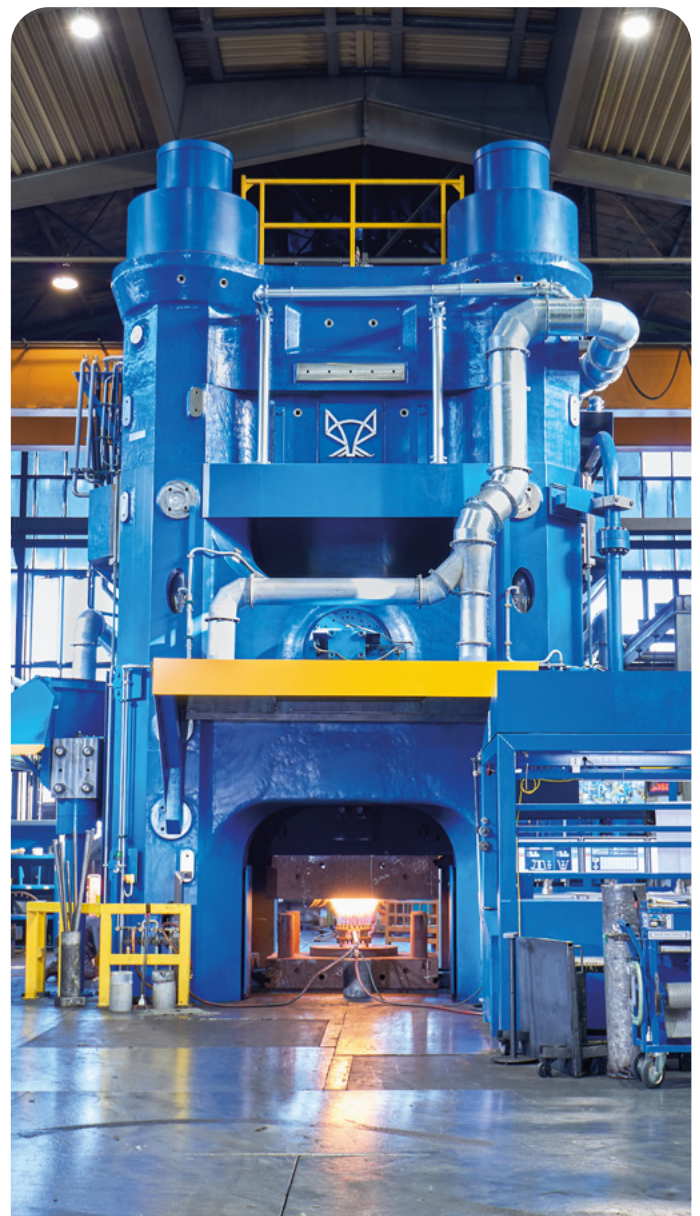
→ Hydraulic forging press (pressing force 30,000 t) for the production of large titanium and aluminum structural components and for the production of forged drive discs made from titanium and superalloys, Otto Fuchs
